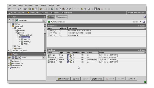
Single or multiple Asd devices can be added as device by selecting the discovered row(s) in the top pane, and clicking add. Doing so will cause the "Add" dialog box to appear:
