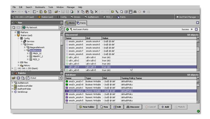
Single or multiple points can be added as control points with AsdProxyExt extensions by selecting the discovered row(s) in the top pane, and clicking add. Doing so will cause the "Add" dialog box to appear: Once the point(s) are satisfactorily edited, click "OK" to create the proxy points corresponding to the point property.
