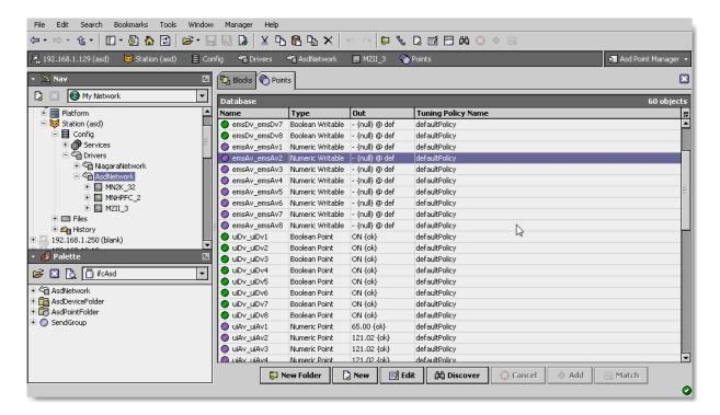
The "New Folder", "New", and "Edit" buttons are not unique to the Asd Device Manager, and are explained in the "Niagara N4 User's Guide" in the "Driver Architecture" section. The "Match" button is not used for the Asd driver.
