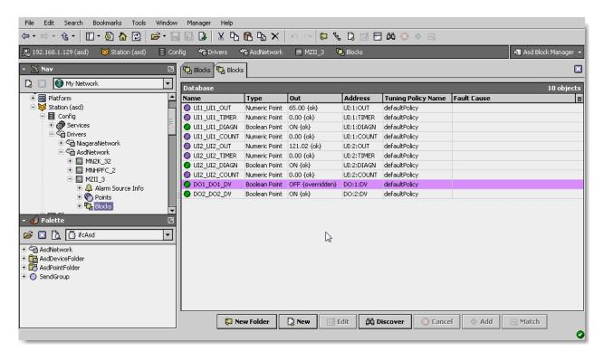
The "New Folder", "New", and "Edit" buttons are not unique to the Asd Device Manager, and are explained in the "Niagara N4 User's Guide" in the "Driver Architecture" section. The "Match" button is not used for the Asd driver.
