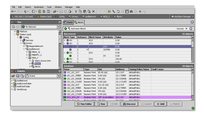
Single or multiple blocks can be added as control points with AsdBlockProxyExt extensions by selecting the discovered row(s) in the top pane, and clicking add. Doing so will cause the "Add" dialog box to appear:
